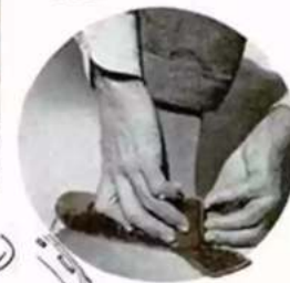
The heel tabs are cut and fitted until the moccasin conforms smoothly to the foot
