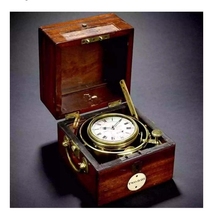
In the pursuit of conquering the seas, sailors confronted a formidable challenge: determining longitude accurately. Enter the marine chronometer, a groundbreaking invention by John Harrison. This navigation instrument accurately measured time, enabling sailors to calculate their precise longitude at sea, revolutionizing navigation in moments perilous and unknown.
